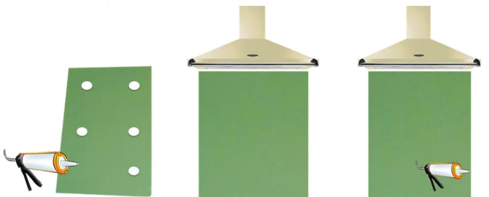
Lay your glass glass side down on a clear surface. Lay a towel or blanket over the work surface to avoid scratching your glass. On the matt side, apply equally sized blobs (roughly 20mm about 100mm apart). Be careful not to put any blobs too close to the edge.
